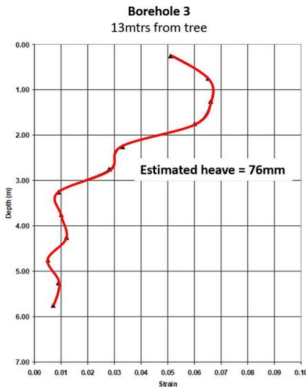
In August 2022, precise levels revealed the station had subsided 64.5mm from the starting point in May 2006, delivering a revised estimate of total heave on rehydration of around 140mm – the area of maximum potential recovery is around 13mtrs from the tree – close to its height.
