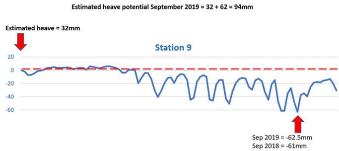
Maximum subsidence of 121.3mm has been recorded at Station 25, 21mtrs from the tree in an adjoining array. In summary, soil tests in May 2006 revealed higher levels of desiccation closer to the tree, dissipating with distance towards the root periphery. There has been a general pattern of recovery closer to the tree, and increased subsidence towards the root periphery. The ground 13m from the tree (nearly matching its height) shows the maximum potential for movement of 140mm.
