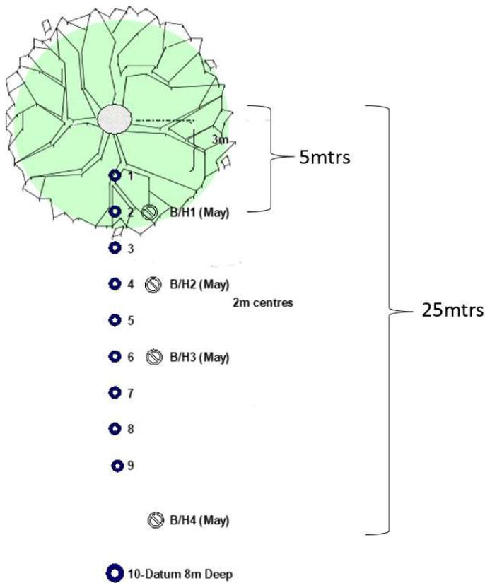
Left, a plan showing the location of level stations 1 – 10 (station 10 is the 8m deep datum) established in May 2006.
